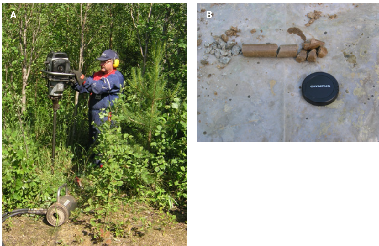
Figure 8. A. Sampling by percussion drilling. B. Soapstone sample taken by percussion drilling. Diameter of the lens cover is 0.5 dm. Photos: Heikki Pirinen.
